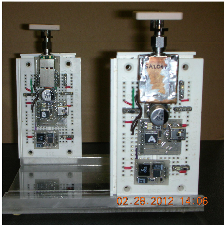
Figure 7 Stock LINX GPS configuration on left, CleanSignal™ Chipset Enhancement on the right
