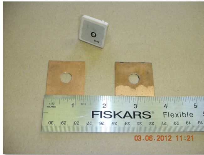
Figure 8 Antenna backplanes used in testing – 1 1/4” x 1 1/4” Copper (left side) and CleanSignal™ (right side)
