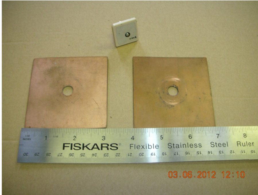
Figure 6 Antenna backplanes used in testing – 3” x 3” Copper (left side) and CleanSignal™ (right side)
